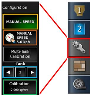
From the **Configuration panel**, select “**Manual Speed**” and confirm that the **manual speed** is set correctly for the operation.
