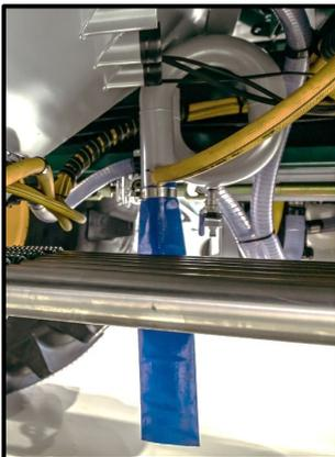
This pipe serves two purposes, the first as the overflow to avoid highly corrosive fluids coming into contact with the chassis etc, and also as a breather for the tank to allow air to pass out of the tank when filling and enter back into the tank when emptying. To avoid contamination the tube is fabricated into an 'S Bend' that forms a fluid filter for the tank.
