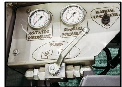
When the pump sucks a large amount of air (for example when the tank is empty), this can also trigger the flow limiting valve.
