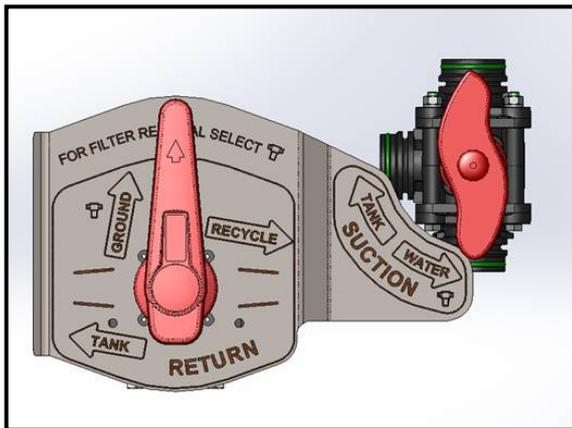
**Suction & Return Valves correctly set for filter servicing**
