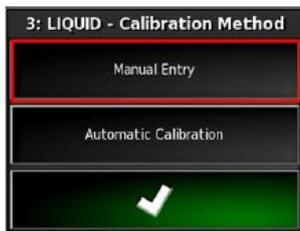
If the product is new or does not have a calibration factor set, select “**Manual Entry**”, and enter a calibration factor of **600 pulses/litre**, and confirm.
