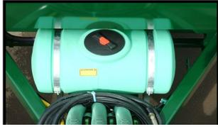
A separate clean water flush tank is provided in order to have ready access for rinse and flush cycles.
