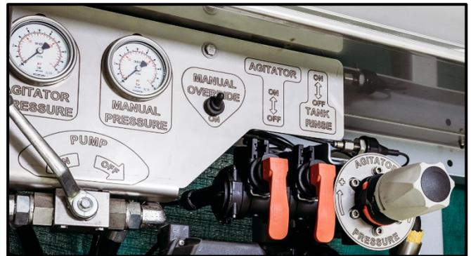
Different agitators are available for differing uses. Simplicity fits the 2.5mm orifice as standard. With this orifice fitted the agitator will roll 600 litres of tank mix every minute if pressure set at 5 bar, or 72.5psi. At this setting the agitator is only drawing approximately 7 litres per minute from the pump.
