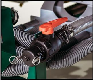
Filling is done via a 2 inch camlock that allows the operator to connect the Air Seeder to an external source and simply pump the fluid in via an external pump. It is recommended that additional filtration be considered so as to avoid any contaminants from entering the main supply tank.
