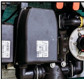
Once through the pressure filter, flow enters the dump valve. The dump valve works inversely to the Section or delivery valve, so when the section valve is closed, dump valve is open back to the return circuit, allowing all pressure flow back to the return circuit.
